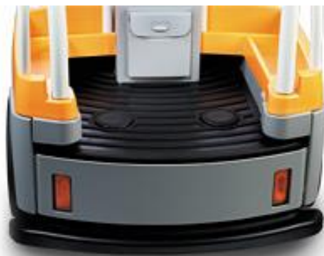
11-12" Step Height, Dual Foot Switch Narrow Operators Compartment
