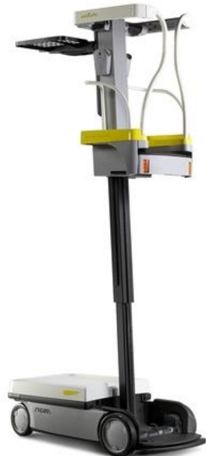
Crown: Telescoping Monomast Gate Behind Operator Design
