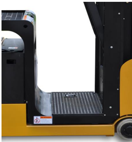
Low 9.5" Step Height, Single Foot Switch Full Width Operators Compartment
