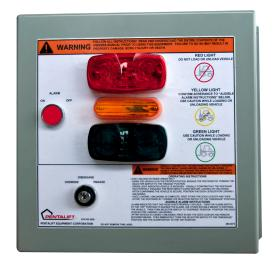
NEMA 12 interior wall mount control station. High visibility interior signal lights are coordinated with exterior signal lights. Clear, concise and easy to follow instructions guide dock attendant on how to use the system. Selector switch and amber light accommodate "override" mode. CSA certified for the design and manufacturer of industrial control equipment.
