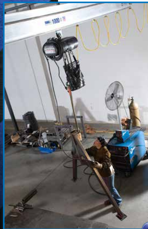
A female worker uses a 1000-pound capacity Spanco Alu-Track Bridge Crane to position product in her work area.
