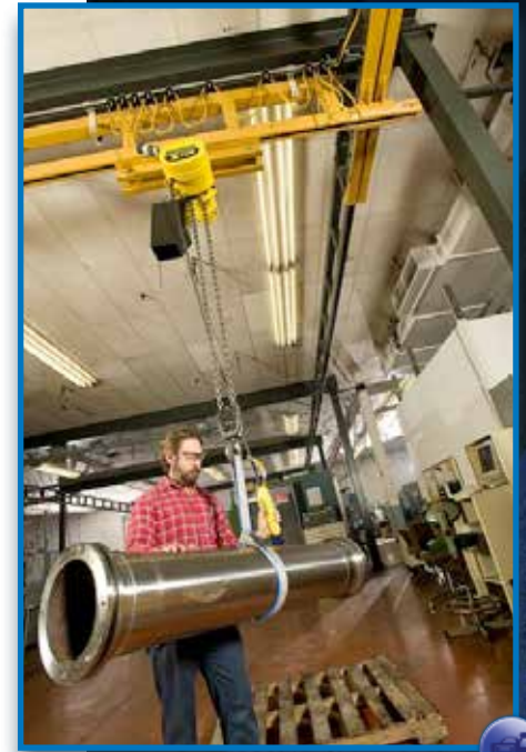
A 4000-pound capacity Spanco Freestanding Bridge Crane carefully lifts and moves an expensive machined part.
