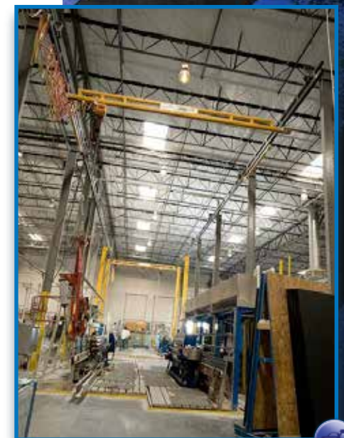
A custom-engineered 2000-pound capacity Spanco Freestanding Bridge Crane for a glass manufacturer.
